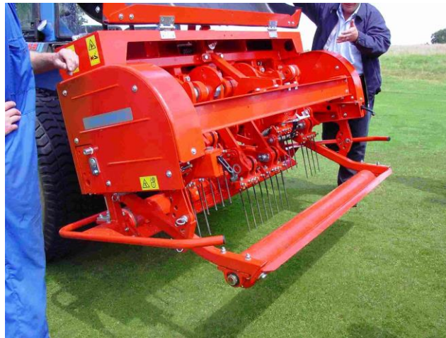
Figure 4-2 Verti drain with 12 mm tines
