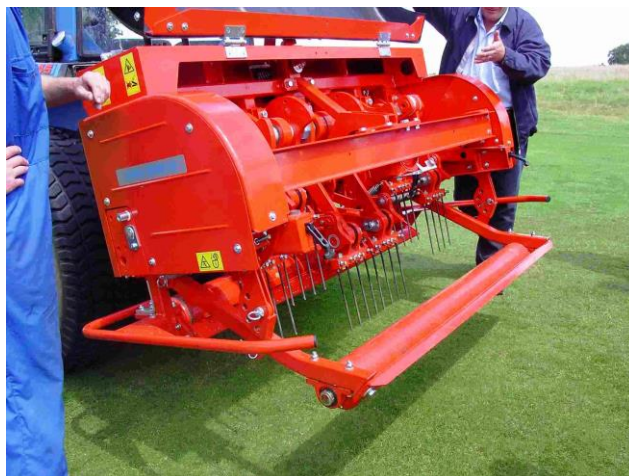
Figure 5-2 Verti drain with 12 mm tines
