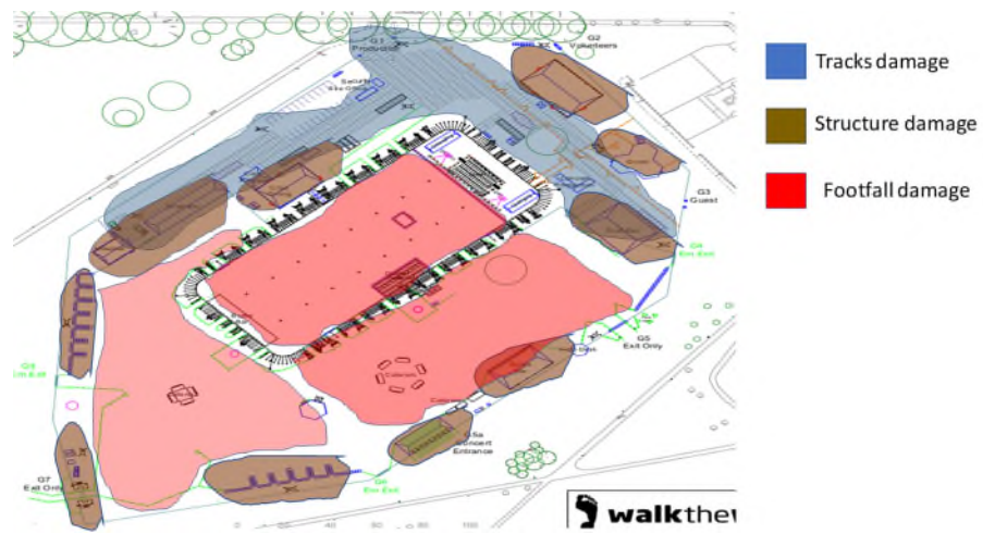
Figure 3-2 Likely areas with different kind of damage to the grass cover
